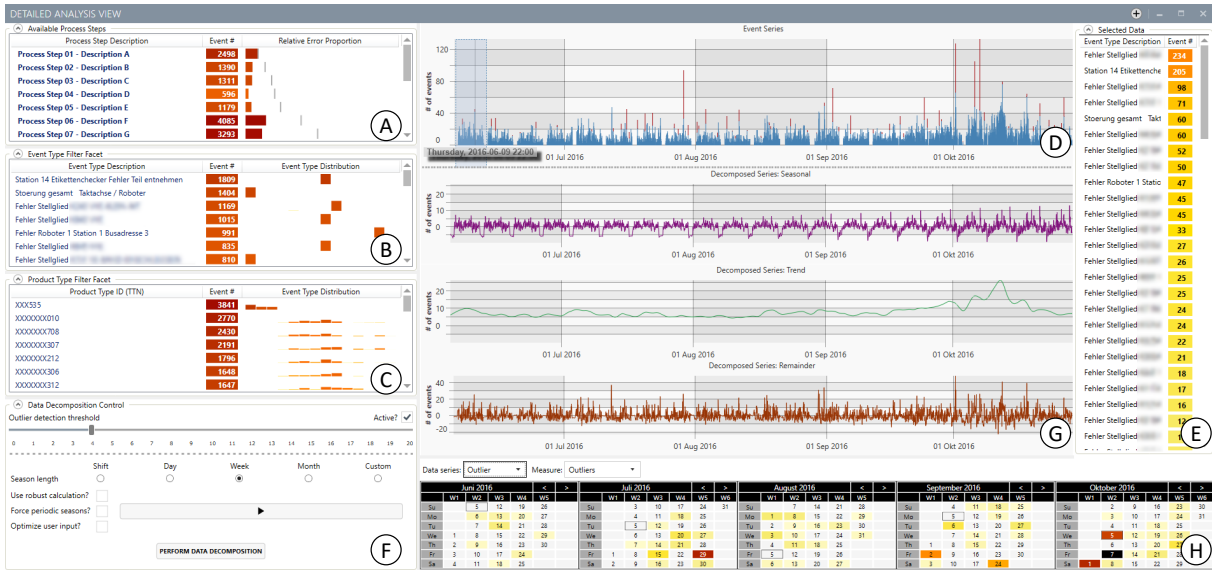
Figure 1: The facet views (A)-(C) on the left provide a first overview of the reported events’ distribution along the production line. The filtered events’ temporal distribution and optionally its outliers are presented as a stacked bar chart (D). Through brushing, analysts can get more information about the reported events during the selected timespan (E). The event series can be decomposed with STL to find recurring events and trends. The decomposition parameters are set in the Data Decomposition Control (F) and its results shown as three line charts (G). The Calendar Plot (H) provides information about outlier or value distributions of the data.
